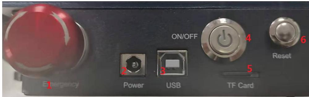
1. Emergency stop switch: In case of emergencies, the machine will immediately stop working when you press it. When you need to unlock it, turn the button clockwise to restart the engraver.
