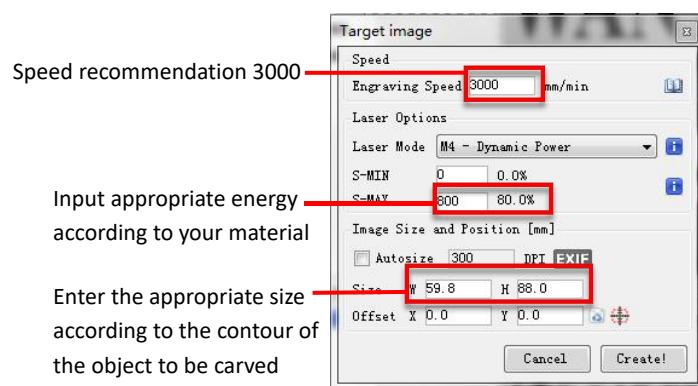
Setting of engraving speed and laser power
