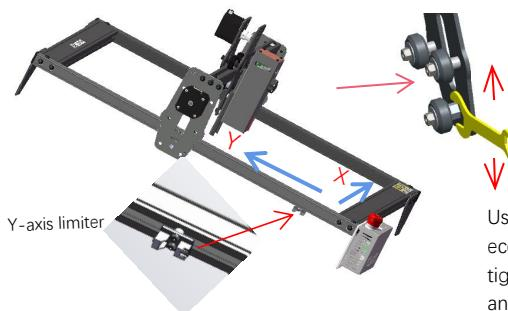
Use a wrench to turn the eccentric nut to adjust the tightness of the guide wheel and the guide rail
