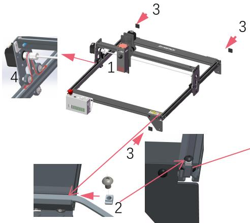
Install the belt as shown.Tighten the T nut and cut off the excess belt.
