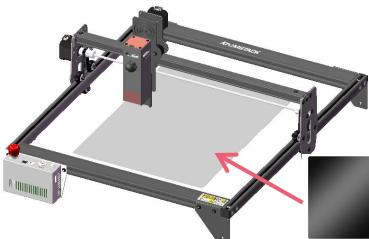
1. As shown in the picture, place the cutting pad under the engraved/cut object
