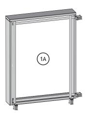
**Example:** Panel (using  $8" \times 8"$  block) is fourteen block wide ( $8 \times 14 + 1/2" = 112-1/2"$ ) and ten block high ( $8 \times 10 + 1/2" = 80-1/2"$ ). Rough opening needs to be 112-1/2" wide and 80-1/2" high.
