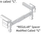
• Where glass block meet the jambs and curb, (except for the four corners) orient the spacer with the cross arm down and clip off the upper set of toothed legs, and the upper half of the twist-off tab.
