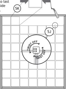
K. Install two blocks, buttering both vertical sides of the second block before installing.
