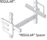
• For the two bottom corners of the panel, orient the spacer with the cross arm down and clip off the upper toothed legs. Clip off the upper half of the twist-off tabs. Cut off the left or right side of the remaining twist-off tab and the smooth legs on the same side. Only two of these spacers are required. Clip off the right set of smooth legs of one spacer, the left set of the other spacer. These are called "L".
