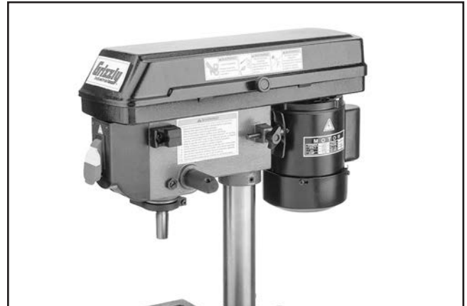
Figure 11. Headstock placed on column.
