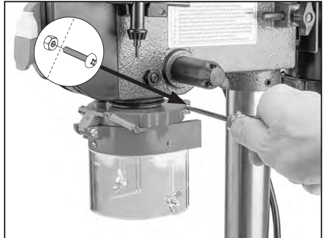
Figure 7. Attaching chuck guard to quill.
