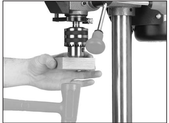
Figure 14. Example of using block of wood and hammer to tap chuck onto spindle taper.
