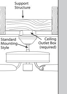
Use Standard Mounting or Low-Profile Mounting to hang the fan from a flat ceiling. **Ceiling Bracket**
