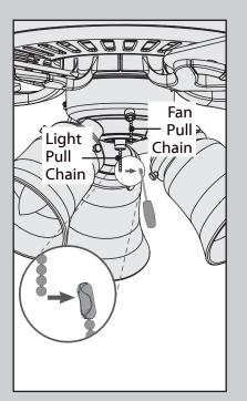
Connect the appropriate pull chain pendant to each of the short chains coming from the switch housing.
