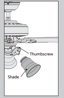
To install the shade, first loosen the thumbscrews. Raise the shade to the light fixture. Tighten all thumbscrews securely. Bulb
