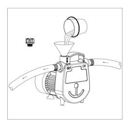
5. For normal water transfer applications, plug in power cord to grounded outlet. Then press the switch on the top of the motor (B), Pump will prime in a few minutes, depending on suction line length.
