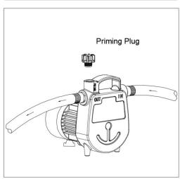
4. Fill pump housing with clean water. Reinstall plug.
