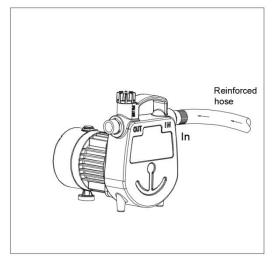
Attach a standard 3/4" garden hose to the OUTLET on the pump. Keep the total length of hose as short as possible for best performance. Secure the hose to keep it from moving around.
