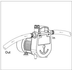
3. Remove priming plug from the top of the pump.
