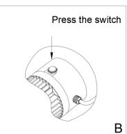
6. If the pump does not pump water after two minutes, turn off the pump and repeat steps 4 through 6. **DO NOT RUN DRY.**
