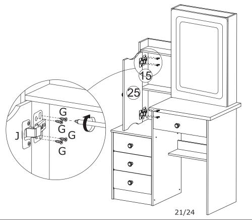
Attach door plate 25 to plate 15 by fixing hinge using screw(G) as shown.
