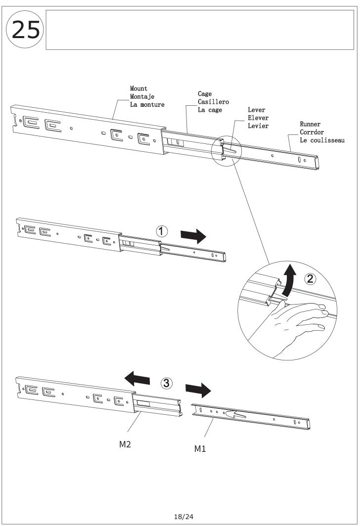
Separate glide into two parts at first.
