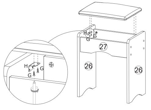
Attach seat plate and fix with iron sheet using screw(G) as shown.
