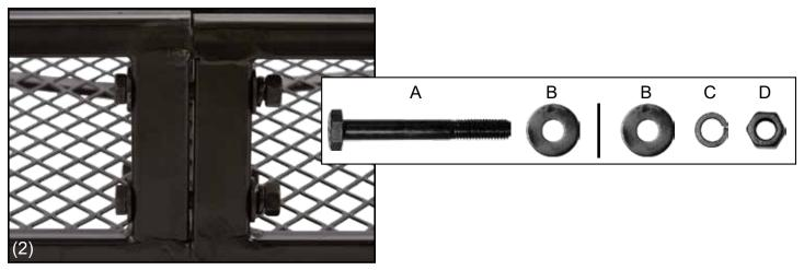
**Step 3.** Flip the carrier over to install the main tube (H). Secure with three M10x80 bolts (A), washers (B), lock washers (C), and nuts (D).
