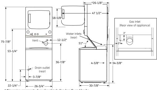
\* Dimension represents door closed including handle and knobs. NOTE: With feet set at mid position, feet can be adjusted +/- 3/8".
