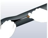
2. With a sharp, non-serrated knife slit the tube along the entire length. When slitting the tube take care not to cut through opposite side of wall.
