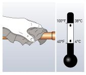
1. Clean all dust, dirt, oil and water from pipework using denatured alcohol where necessary. Install Tubolit when ambient temperature is between 40°F (4°C) and 100°F (38°C).
