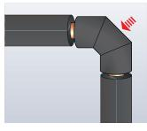
6. For soldered or welded pipes, insulate the fittings first followed by the straight sections.
