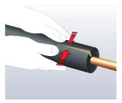
5. Free the seams from the pipe where applicable. align the edges and press the seam detail with firm, even pressure to finish.
