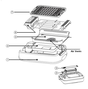
First, Turn the appliance over , put the fan motors at the bottom see Part 1. 2. 3. Second , put water(oil) collection tray in the bottom see Part 4. Third,Put the heating -insulation plate in see Part 5
