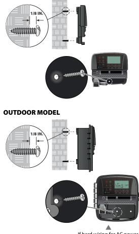
If hard wiring for AC power, remove knockout for conduit
