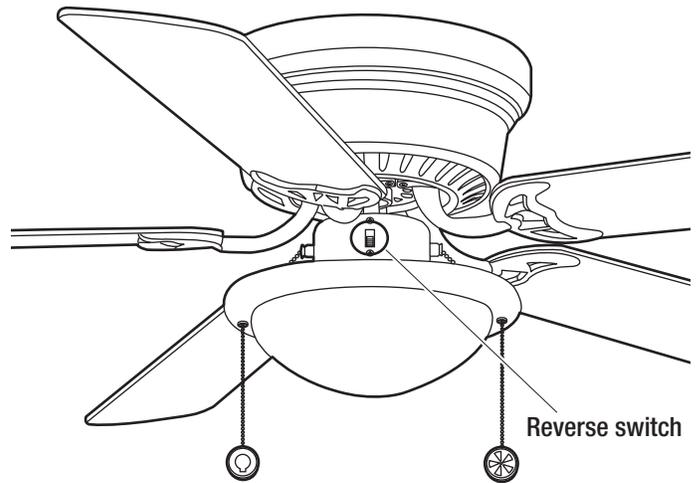
**Warm weather - (Counterclockwise Direction)** A downward air flow creates a cooling effect. This allows you to set your air conditioner on a warmer setting without affecting your comfort.
