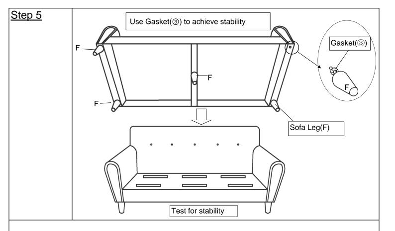
Install the Sofa Leg(F) at the base of the Sofa by placing one Gasket(③) on the threaded stem. Then insert threaded stem into the threaded mounting postion at the corner of the Sofa.
