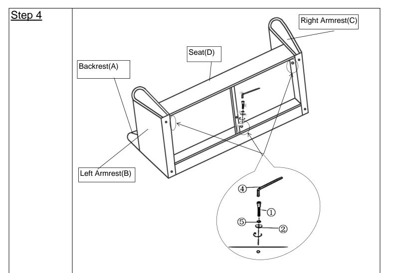
Tilt and lay the Sofa on its Backrest(A) onto a flat surface.
