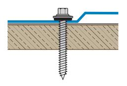
1. The tip of the screw is made for the deck underneath.
