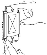
Align control and tighten screws.
