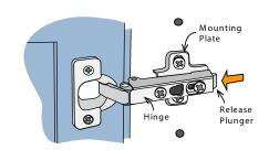
To Remove a Mounted Hinge:
