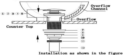
Vessel Sink/Drain Installation(non-Overflow)
