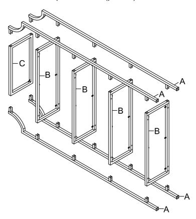
Step 2. Attach top shelf frame(part#C) and shelf frames(part#B) to the legs(part#A) by using bolts (part#1) and allen wrench(part#2). Bolts(part#1) will be inserted from the opposite direction for top shelf frame(part#C) only.
