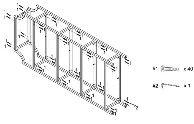
Step 3. Carefully turn unit upright.Install glass shelves(part#D) and top glass shelf(part#E) into the frame as shown below.
