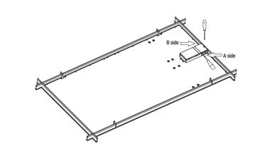
Place the LED flat panel fixture into ceiling and ensure the power supply is off.
