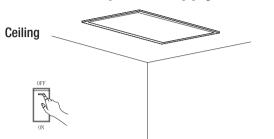
Fix the flat panel fixture on the T bar grid in the ceiling by twisting 4 pcs of T bar grid clips onto the bar.
