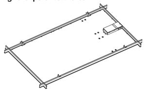
Remove the cover of junction box on the back of the fixture with a screwdriver. Remove the knockouts on the A and B side with a screwdriver.
