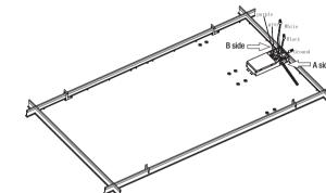
Attach the junction box cover plate on the LED Flat Panel fixture with the screw using a screw driver. Turn on the power supply.
