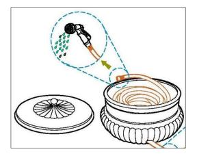
3. Keep the spray nozzle at the top or in an accessible location before closing the hose pot.
