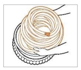
1. Insert the female end of the garden hose through the hole at the bottom inside the hose pot.
