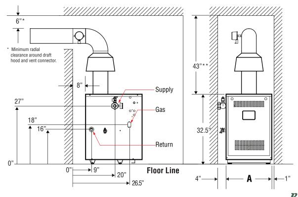
\*\* Additional height required to maintain 6" clearance from all vent connector components. Vent damper may be installed in vertical or horizontal section of vent connector within reach of vent damper harness.
