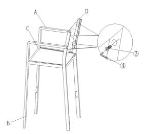
Attach Backrest(D) between Right Leg(B) and Left Leg(A) using Bolts(3) with Allen Key(4) as shown above.
