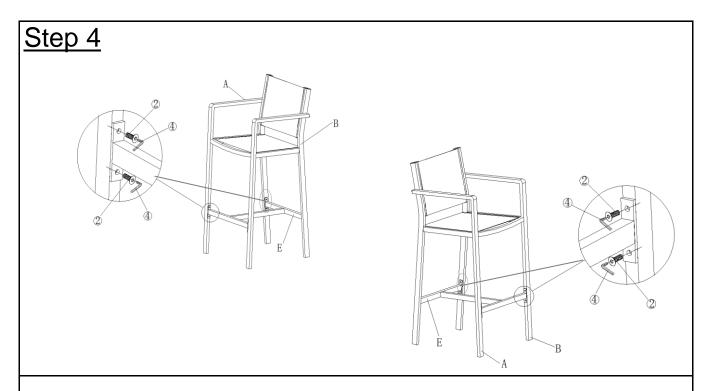
Attach Footrest(E) between Right Leg(B) and Left Leg(A) using Bolts(②) with Allen Key(④) as shown above.
