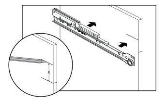
Mark "X" from front bottom mark. Align top of Cabinet Side Slide with mark.
