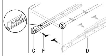
To install Drawer ④ into Cabinet ③ make sure the Soft Close Damper is pulled foward (as shown in ⑤) then push drawer in until Soft Close Damper catches and pulls the drawer closed.
