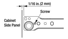
Line up slides to your marks in the cabinet and ensure Cabinet Side Slide Left (C) and Cabinet Side Slide Right (D) are level. Then attach with 3 screws (F) to each side.
