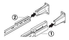
Ensure each Cabinet Side Slide ② and ① is level and attach with two screws (F) to Face Frame Cabinet.
