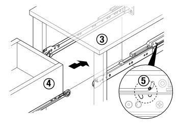
Once drawer is installed, check drawer alignment to ensure the soft close damper is engaging. If necessary, remove drawer and adjust rear panel brackets as needed. Once final placement is achieved, remove drawer one last time and secure rear panel brackets with remaining screws from SKU 1002772986.
