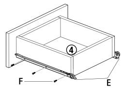
To install Drawer 4 into Cabinet 3 make sure the Soft Close Damper is pulled foward (as shown in 5) then push drawer in until Soft Close Damper catches and pulls the drawer closed.
