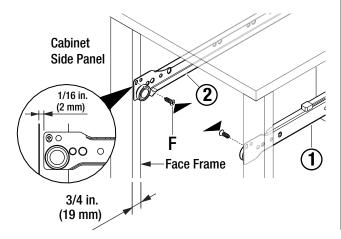
Ensure each Cabinet Slide ② and ① is level and secure bracket to back of cabinet with 2 screws provided in SKU 1002772986.
