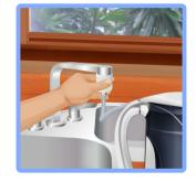
Keeping outer ring in the down position ,place connector under the faucet and push it up onto the faucet to fit securely in place.
