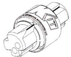
Insert stripped wires into opposing ends of connector. When properly inserted the wires insulation will be inserted into the housing approximately ¼".
