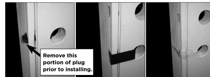
FIGURE 4: Some door units may be supplied with a "clip" or "plug" holding the panel aligned and closed during the initial installation steps. Do not remove at this time. Some door units may be supplied with a double headed nail or screw holding panel closed - this needs to be removed at this time.
