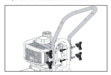
Attach the left handle and right handle to the middle handle using the knob nuts, lock washers, flat washers and curved head bolts provided. The knob nuts should be on the outside.
