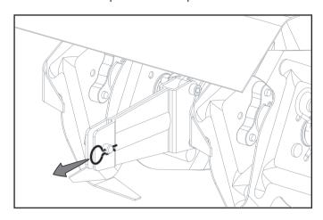
2. Remove the clevis pin from the axle assembly.
