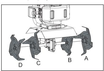
3. Insert the R clip into the holes at each end of the tine shaft to lock the tines into place.
