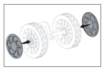
6. Attach wheel assembly to main body, reverse steps 1-2.
