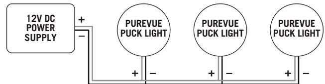
On very large, multi-LED light installations, be aware of possible voltage drop, which only becomes undesirable if you notice the brightness in one area of your lighting is objectionably different than in another area. Do not coil wire; shorter lengths and thicker wire will mean less voltage drop and higher brightness. For an online voltage drop calculator, visit [armcastlighting.com/voltagedrop](http://armcastlighting.com/voltagedrop).
