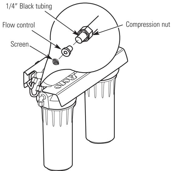
**14** Turn on water supply. Allow to fill. (May take up to four hours.) **Check for leaks.**
