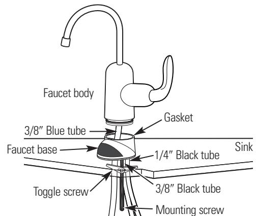
7. Push the faucet body down into the faucet base and twist clockwise until it stops into place.
