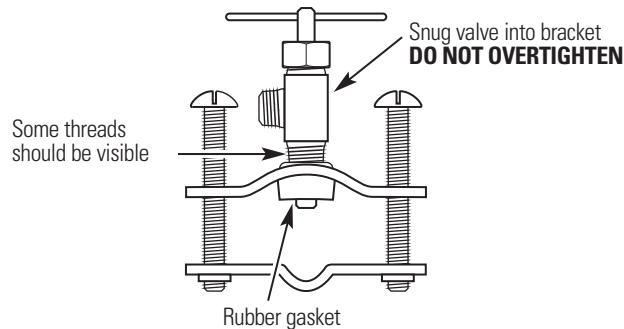
Optional water supply connection (using saddle valve)\*
