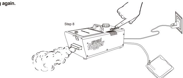
Step 8: Manual Activation: Simply press and hold the "Manual Activation Switch" to ON located on the top of the ground fog machine. The ground fog machine will spray fog for 30~50 seconds. Release the switch to return to OFF position. The machine will automatically stop when it needs to reheat, Wait for the preheat red light to come on before operating again.
