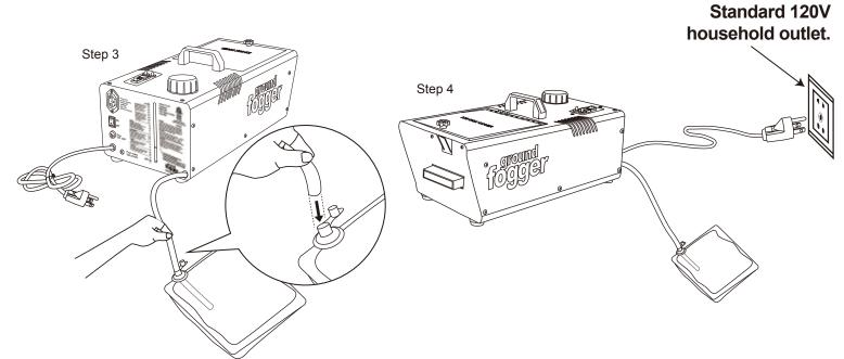
Step 3: Open the cap on the water bag plug and insert the water tube into the water bag. When ice melts into water, water will flow into the water bag.
