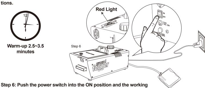
light will illuminate. Allow the machine to warm-up 2.5~3.5 minutes.
