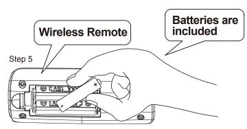
Step 5: Open battery cover on back of wireless remote. Insert the new 2 X 1.5 V AAA batteries inside. Please observe the correct polarities during installation and follow all battery instruc-
