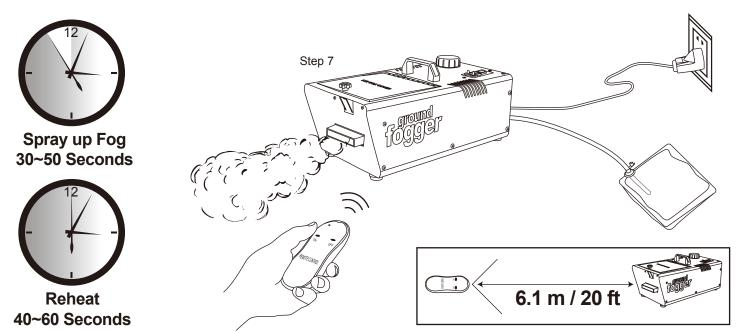
Step 7: Wireless Remote Activation: Point wireless remote towards the wireless receiver dome located on top of the ground fog machine. Press the "ON" button and the ground fog machine will spray fog 30~50 seconds. Press the "OFF" button to stop. The machine will automatically stop when it needs to reheat. Wait for the preheat red light to come on before operating again.
