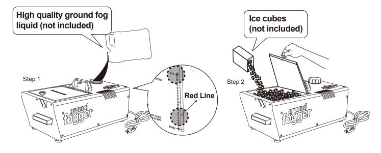
Step 1: Remove the cap of the fluid tank to fill with high quality ground fog liquid. NOTE: THE AMOUNT OF FLUID CANNOT EXCEED THE "FULL" MARK ON LEVEL INDICATOR. PLEASE ADD GROUND FOG LIQUID WHEN THE AMOUNT OF LIQUID IN THE "RED LINE" MARK ON LEVEL INDICATOR.
