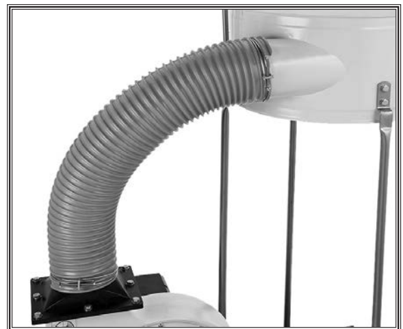
Figure 14. Transfer hose attached.
