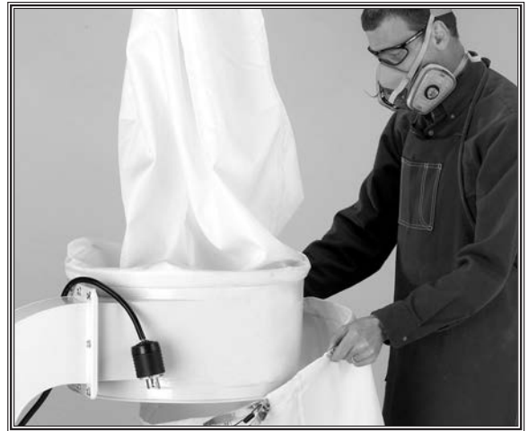
Figure 38. Replacing lower bag.
