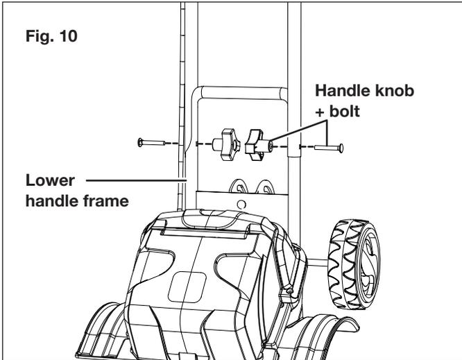
**NOTE:** Make sure that the handle knobs are placed inside the handle frame. Otherwise they will affect the wheel adjustment system.
