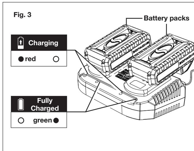
4. When the charger lights turn green, the batteries are fully charged (Fig. 3).
