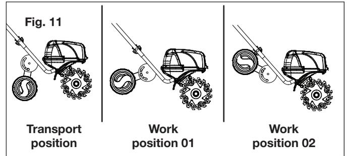
2. To adjust the wheel position, push the wheel adjustment knob while moving it to the slot for desired position; let go of the knob and make sure it locks into position (Fig. 12).
