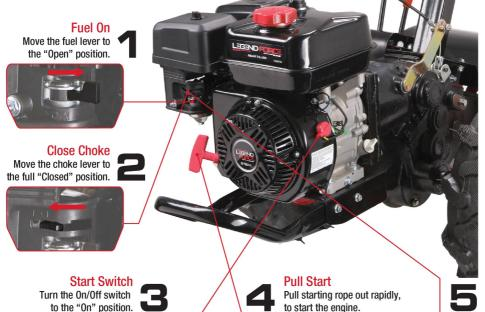
NOTE: Restarting an engine that is already warm from previous running does not normally require use of the choke.
