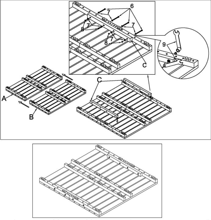
Turn footplates part (A) and part (B) facing down, forming a trapezium shape. Affix the Wood Cleat (C) along the inner side of the trapezium border. By aligning the threaded holes, place the washer (7) around the bolt (6), insert bolt from the outside through the border and wood cleat, secure with a washer (7) from inside of wood cleat, followed by a nut (8). Tighten with wrench (9). Repeat same steps for the other side.
