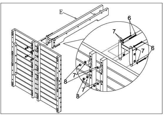
Put the footplate vertically upright and the lower pole (E) laying horizontally with the arc shape facing upwards. Align the threaded holes on the footplate with the hardware holes on lower pole (E), place the metal washer (7) around the bolt (6), insert bolt from the lower pole through the hardware hole to the footplate, secure with a washer (7) from bottom of footplate, followed by a nut (8). Tighten with wrench (9).
