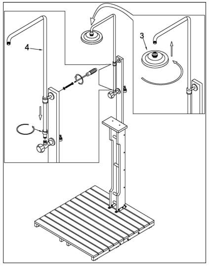
Remove the bolt & washer from the L-shaped pipe (4) holder, position the holder to align with the threaded hole of upper pole (F), then secure with washer, screw into the holder from the back of upper pole (F), tighten with a Phillips screwdriver. Insert the bottom end of the L-shaped pipe into the faucet (1), ensure that the rubber washer is in place before tightened.
