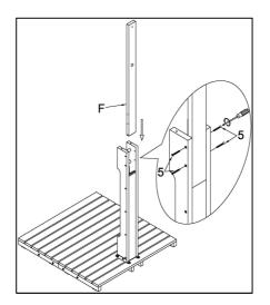
Place the assembled footplate upright. Insert the upper long pole (F) with four threaded holes into the lower pole, secure with screw (5), and tighten with a Phillips screwdriver.
