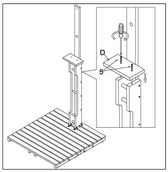
Position the soap holder (D) into the gap at top of lower pole. When in position, secure with screw (5), and tighten with a Phillips screwdriver.
