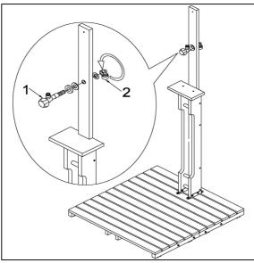
Unbolt the nut of faucet (1) and insert it through upper pole (F), then tighten the nut back on the faucet (1). Be cautious not to drop the metal washer & plastic washer in faucet.
