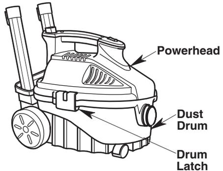
2. Lay the Powerhead upside down on a clean dry area while emptying the Drum or changing the Filter.
