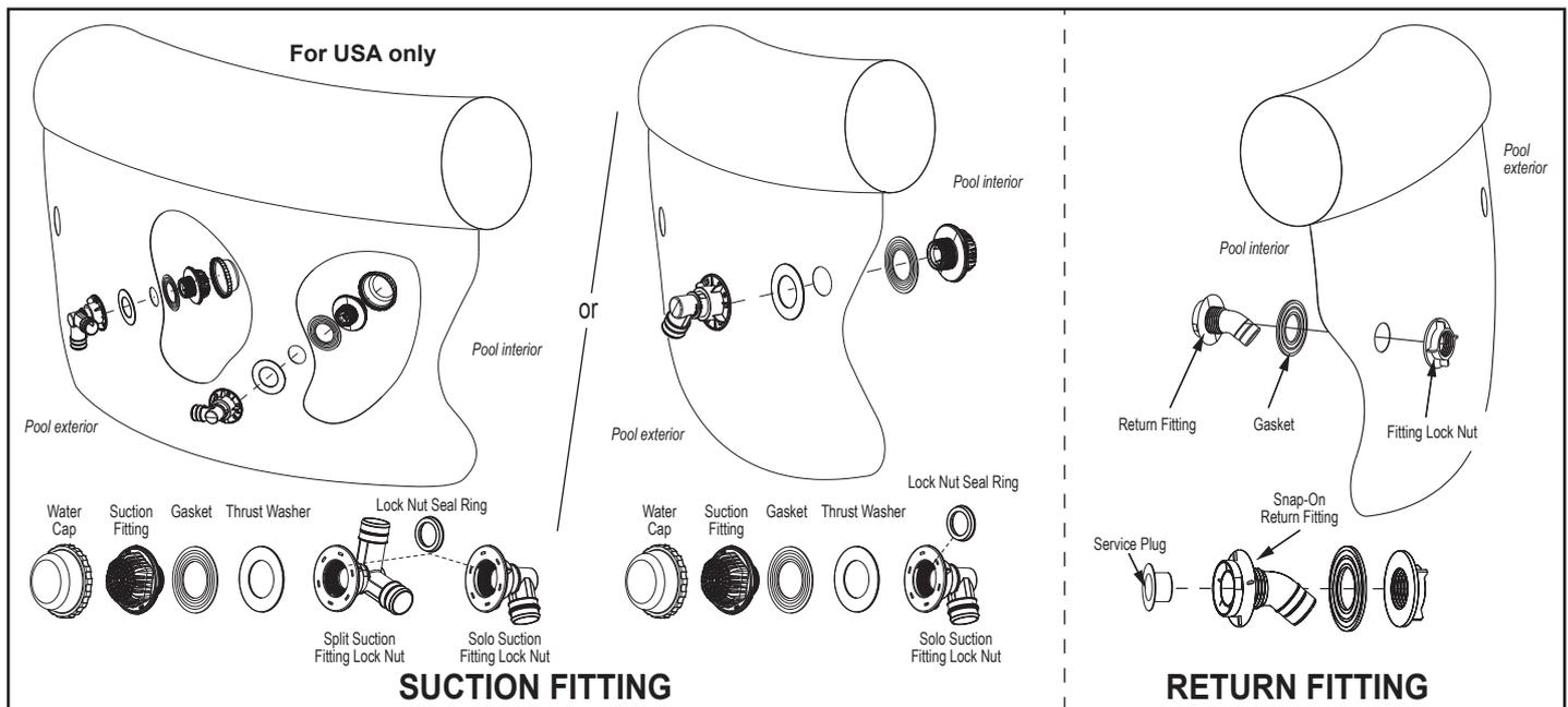
Please Note: The Black Rubber gasket (Gasket) should always be slid over the threaded plastic suction or return fitting and be on the inside before the fitting is placed through the pool wall to make a watertight connection.
