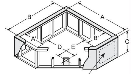
Allow an accessway to the pump/blower (bathtub with system)
