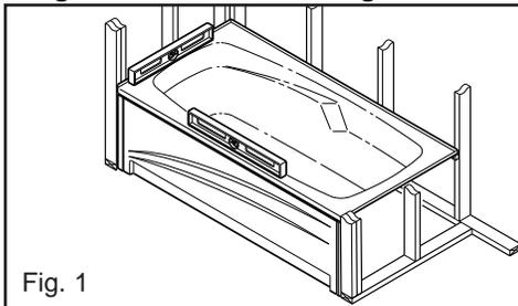
Before installing the unit, the frame and plumbing must be completed in compliance with the instructions. If it is renovation work taking place, the wall surfaces must be removed in order to allow for the installation of the appropriate structural frame.
