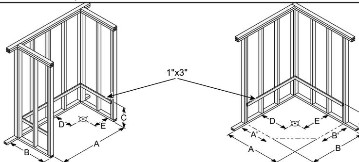
**Note:** The following measurements are not those of the unit but those required for the installation ( $\pm 1/4"$ ); for easier installation add  $1/4"$  (6 mm) to dimensions A and B.
