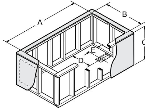
**Note:** the dimensions are for inside, with the exception of dimension «C».
