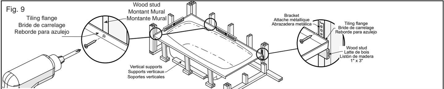
Secure a vertical support in front of the bathtub (leave a space in front of the support so as not to interfere with the installation of the apron, if applicable). Fig. 9. **Make sure the vertical support does not press on the jets or piping.** Incline the support as required to allow easy installation.
