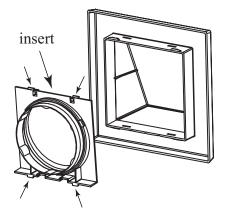
**Step 2** Remove the insert from the trim ring by disengaging the 4 tabs. See figure at left.
