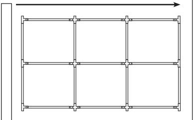
6) Lift the Opposite Side of the Canopy and Attach the Legs and Foot Pads in Same Way. Begin with the Center Legs.
