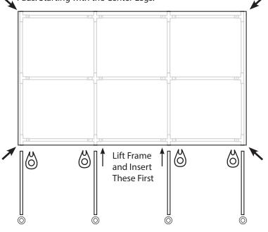
7) Fasten the Drawstring to the C-Clip at Each Corner and Tighten by Pulling the Cord Down and Hooking it on to the C-Clip. Clip the Center Leg Valance Straps to the Cover and Secure Them to the C-Clip. Tighten Them by Pulling Down and Hooking on to the C-Clips.
