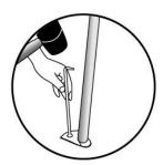
C) To stabilize the canopy,unroll the guy rope on the corner of the canopy. Tie the other end to the stake and then drive the stake into the ground to secure. (Adjust the stake position to tighten up the guy rope.) Repeat for each guy rope.
