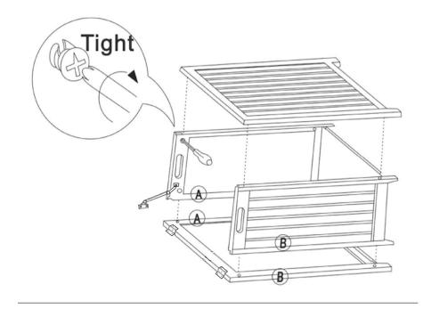
5) Align Hamper Lid to the Back Panel using the four Screws for Hinges provided with a screwdriver to tighten. Connect the Piano Hinge to the Hamper Lid (see diagram) using the two Screws for Piano Hinge with a screwdriver. Insert Interior Bag into the hamper (see diagram). Close the lid and you are done. Congratulations on your new hamper!
