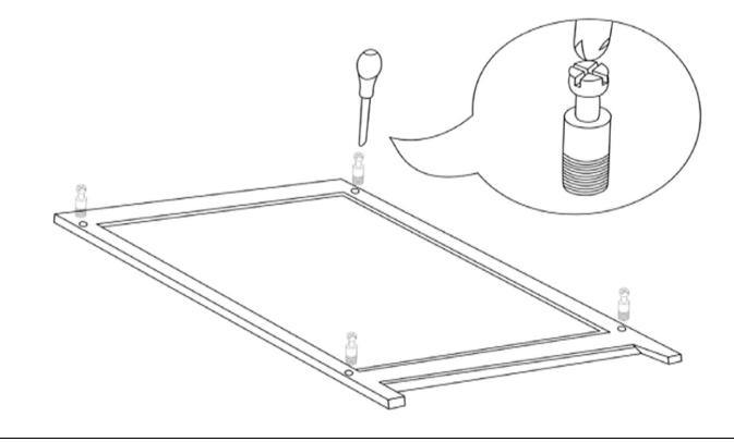
3) Align Right and Left Side Panels to the Back Panel and connect them together. Use a Slotted screwdriver or Phillips screwdriver to tighten the Cam Inserts. Slide the Bottom Board as shown below.
