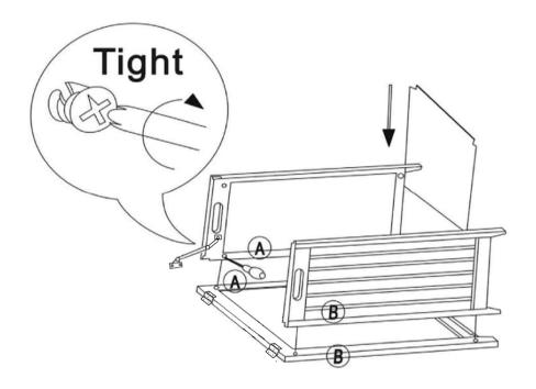
4) Align Front Panel (Flat Style shown below or Bowed Front Style) to the Side Panels and connect them together using a Slotted screwdriver or Phillips screwdriver.
