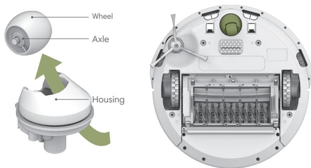
**⚠ Important:** A front wheel clogged with hair and debris could result in floor damage.
