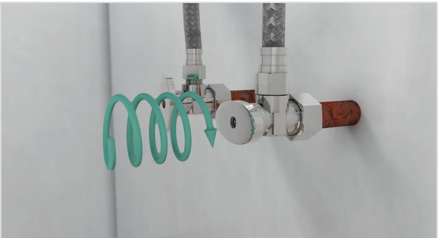
Diagram 2.3(B).4 Shutoff Cold Water Source Valve
