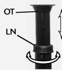
c) Overflow tube (OT) is 1/2" above water line (WL) & at least 1" below flush lever nut (FN). Hand tighten locknut (LN) when done.
