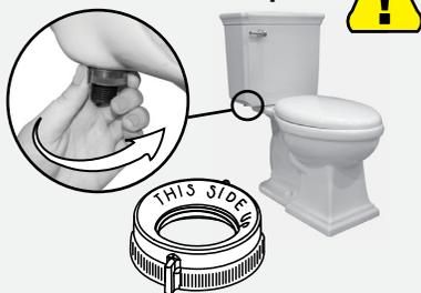
c) Insert metal clip into refill tube.
