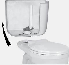
c) Remove sponge gasket. Remove mounting nut (MN) with wrench. Remove valve and hardware.
