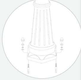
3. Attach the middle pole (F) to the base pole (G) using the three provided screws.
