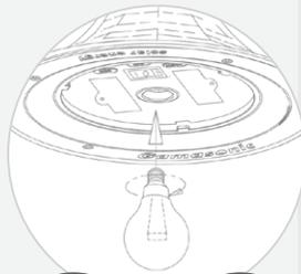
9. Install the lens (H) onto the lamp head (A) by twisting clockwise.
