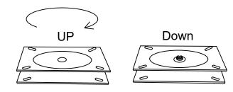
Rotate the top half of component 2 by 45°.
