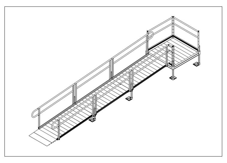
Configuration shown with straight ramp run and 4' x 4' top platform.
