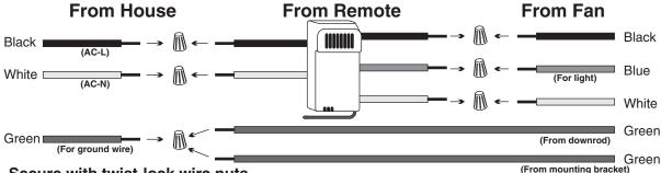
Secure with twist-lock wire nuts.
