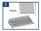
Before installing the first TITAN 3000 measure 2 inches from the end and notch the front and back of the TITAN 3000 Bend remaining 2 inch flap 90 degrees to create an end cap
