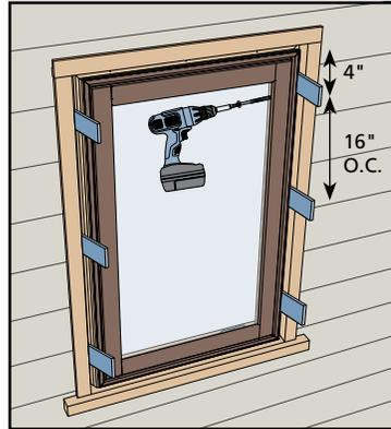
5. Inspect pocket window for plumb, level, and square dimensions. Additionally, evaluate for twist. Correct as needed. See **Product Installation Tolerance Table** for tolerances.
